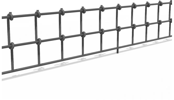
Fence completely made of Ø16 mm steel and 30x6 mm base with reinforced structure treated with Ferrus, a protective process that guarantees high resistance to corrosion.
