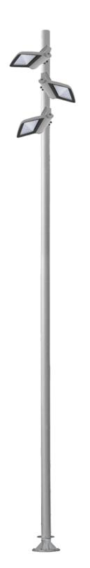
Pole made of S-235-JR hot-dip galvanised steel available in two formats: \*Height up to 8 m for TOP mounting of the luminaire with  $\varnothing$ 60 mm; \*10 and 12 m cylindrical ones are only and exclusively designed for the installation of circular floodlights with outer equipment (can be housed in the 3 service doors available)
